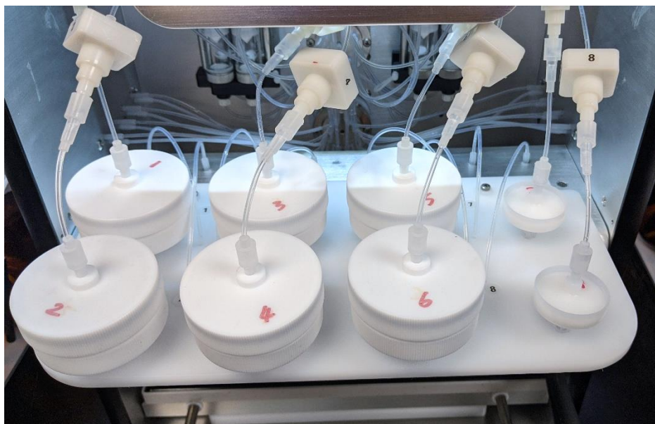
Figure 1 - 47mm Disks and Mini-disks on the SPE-03 Disk Rack
