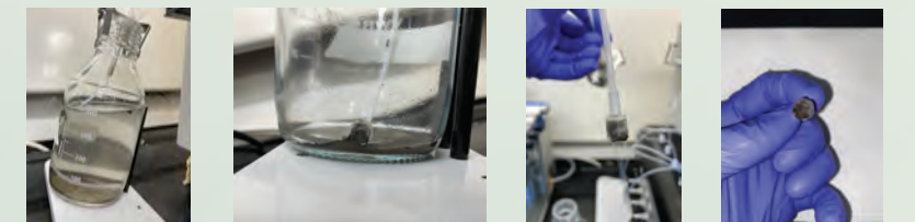
Figure 5 - Using Anti-clogging Tips for seawater samples with sediment and algae
