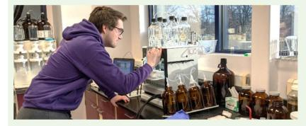
Merit Laboratories had been extracting TCLP SVOCs using 47-mm disks and a vacuum-based extractor, hereon referred to as the "benchmark". To overcome the limitations in sample throughput and variations in extraction time, PromoChrom's MD-BNA-30 Mini-disk and SPE-03 8-Channel extractor were introduced. While 47mm disks require disk holders, the Mini-disks come pre-packaged for direct connection to the SPE-03 or any standard luer connector.
