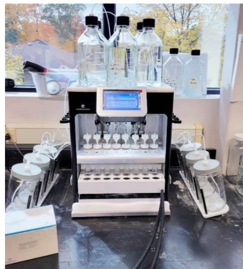
Figure 2 - SPE-03 Setup with Mini-disks which does not require the Disk Rack
