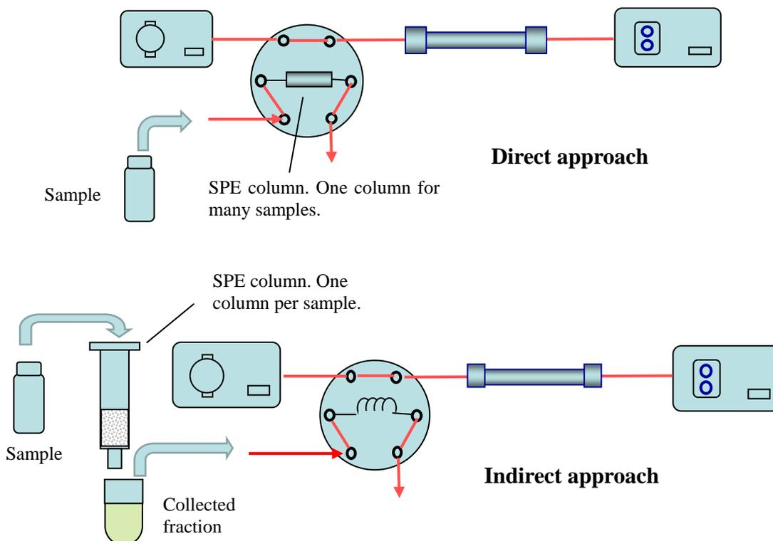
Using the direct approach can achieve high sensitivity and fast sample throughput since the entire cleaned up sample is used for final analysis and the procedure is simple. For example, in the analysis of trace pollutants in drinking water using offline SPE, the sample volume is normally around 500 mL.
