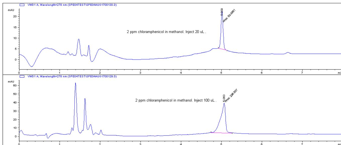
As shown in the above chromatograms, a 20  $\mu\text{L}$  sample volume gave a good peak shape despite the difference in solvent. When the injection volume was increased to 100  $\mu\text{L}$ , the peak broadening
