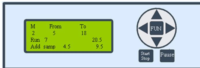
The screen indicates that samples 5 to 18 are to be processed using method 2. It is now performing the add sample action on sample 7. The sample intake is set to 20.5 mL for each sample.
