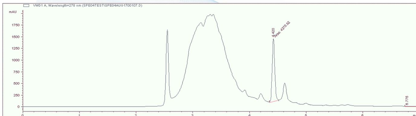
The estimated detection limit based on the peak height is 0.2 ppm. Processing time for one sample is 10 minutes. After 20 samples, the SPE cartridge began to show blockage. The following experiment demonstrates how the two-tier approach can extend SPE cartridge lifetime and improve sensitivity.
