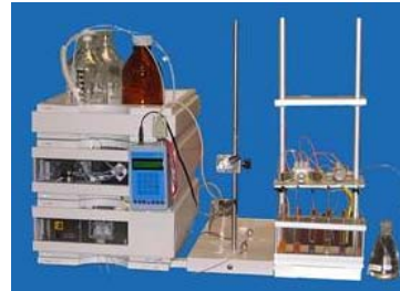
Fig 1. A configuration for GPC cleanup.
